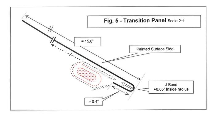
The 4" wide Transition Panel fits over the 1.5 inch gap between the Extension Panels to allow for Panel expansion and also covers the up/down ice melt cable transition loops at each end of the HotShingle™ Extension runs. These cable loops can be run up-roof for additional Panels or down-roof into the gutter or for power feed for a complete heated drain path.
