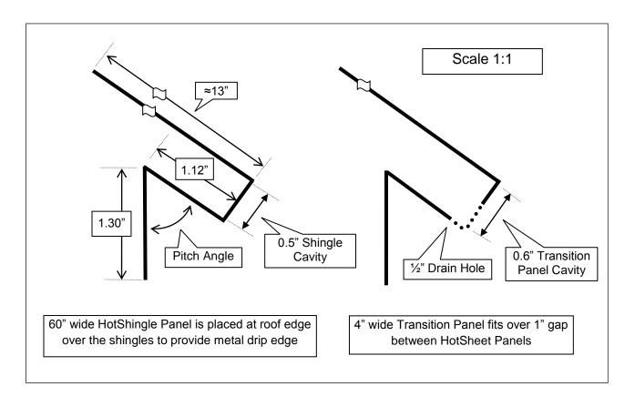
The HotShingle™ Panels are normally five feet wide and installed with a one inch gap for expansion and drainage between the panels. The four inch wide Transition Panel has a slightly larger inside cavity and fits over the gap between the longer HotSheet™ Panels. The ½ inch hole on the underside of the Transition Panel provides continuous drainage path for any water under the panel.
