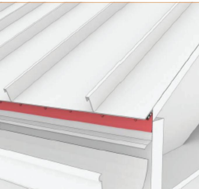
HotEdge Rail is the first and only UL Listed roof edge ice melt system in the U.S. The revolutionary NEW patent-pending HotEdge Rail is engineered to prevent icicles and ice dams from forming along the edge of most roof structures by compressing a 12-watt commercial-grade, self-regulating heat cable directly against the existing metal drip edge. HotEdge Rail fastens to the fascia beneath the metal drip edge of a roof, providing a containment system for the heat cable.
